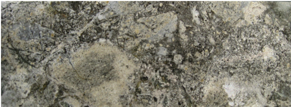
Figure 7.17. Diorite breccia with alteration halos on fragments from hole CV98 at 292 meters (assay interval contains 0.268 grams gold per tonne and 0.120% copper) (Source: Behre Dolbear, 2013)
