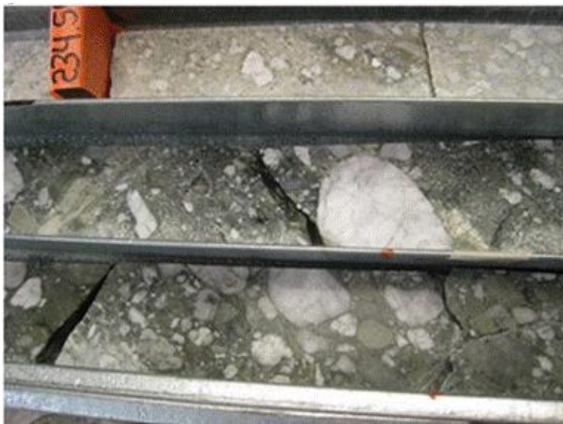
Figure 7.6. Photo of the basal quartz pebble conglomerate of the Amaga from drill hole MJ-6 (Maria Jo) at 234 meters (Source: Behre Dolbear, 2013)
