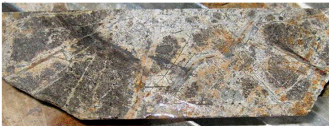
Figure 7.15. Stockwork contact breccia from CV053 at 98 meters (assay interval contains 1.5 grams of gold per tonne and 0.06% copper) (Source: Behre Dolbear, 2012)
