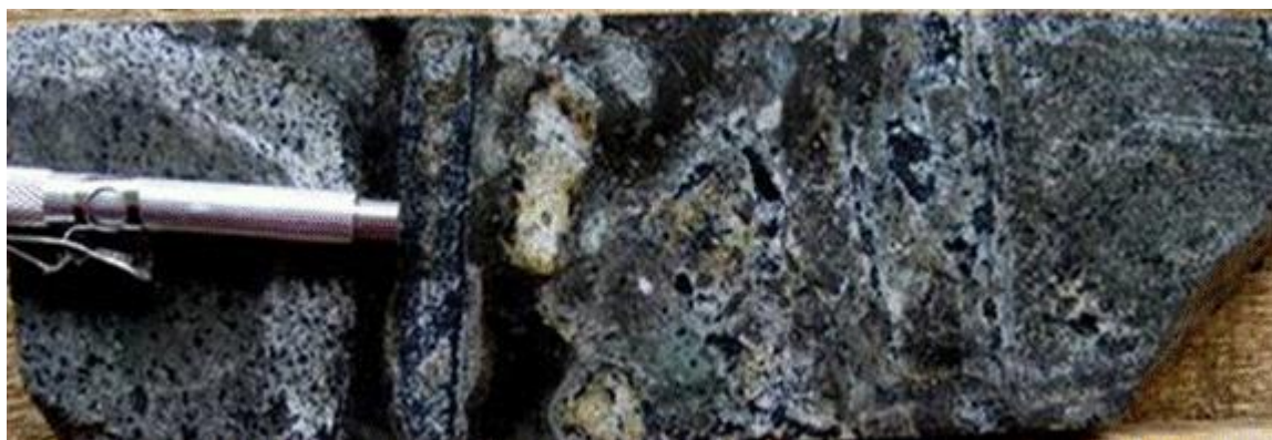
Figure 7.13. Intrusive breccia with magnetite-rich fragments, magnetite-rich matrix from drill hole CV038 at 208 meters (assay interval contains 0.3 grams of gold per tonne and 0.23% copper) (Source: Behre Dolbear, 2011)
