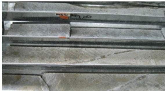
Figure 12.6. CP022 – highlighting a portion of 347.0 meters to 348.5 meters, with obvious pyrite veins (Source: Behre Dolbear, 2013)
