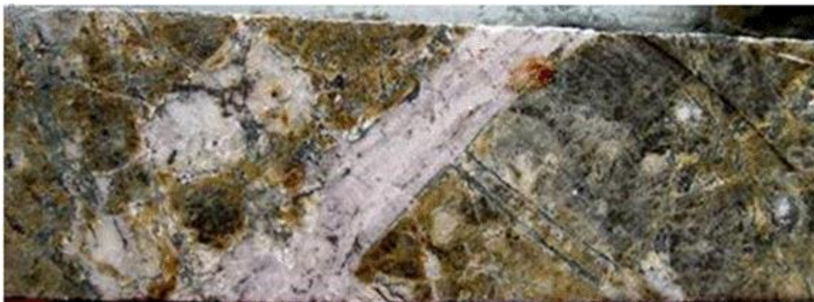
Figure 7.12. Multiple-stage mineralization from drill hole CV018 at 393 meters (assay interval contains 0.5 grams of gold per tonne and 0.25% copper) (Source: Behre Dolbear, 2011)
