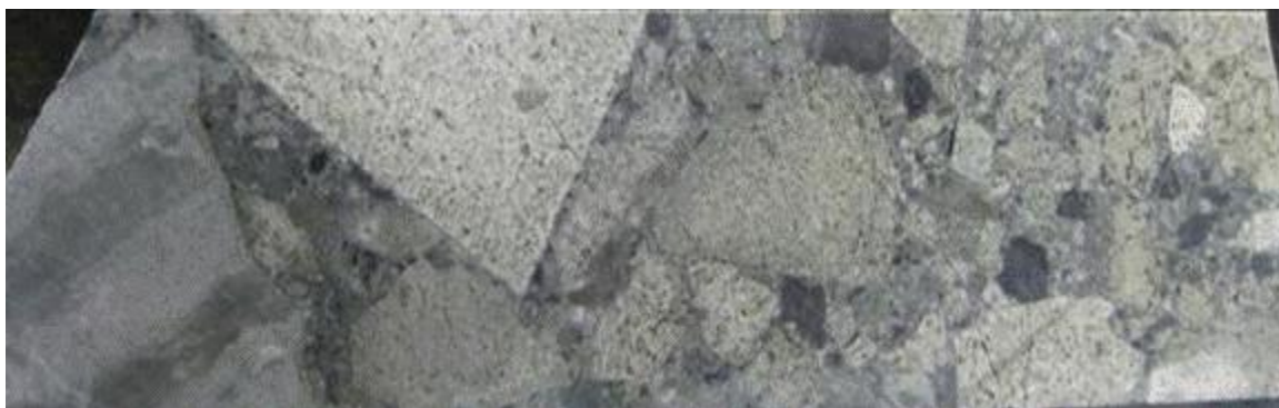
Figure 7.18. Diatreme breccia from CP014 at 29.5 meters (assay interval contains 0.7 grams of gold per tonne) (Source: Behre Dolbear, 2012)
