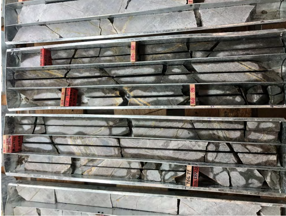
Figure 12-13 ¼-core for duplicate checks ready for sampling as prepared under the supervision of the QP during the current site visit (Source: Mauricio Castañeda, June 12, 2021)
