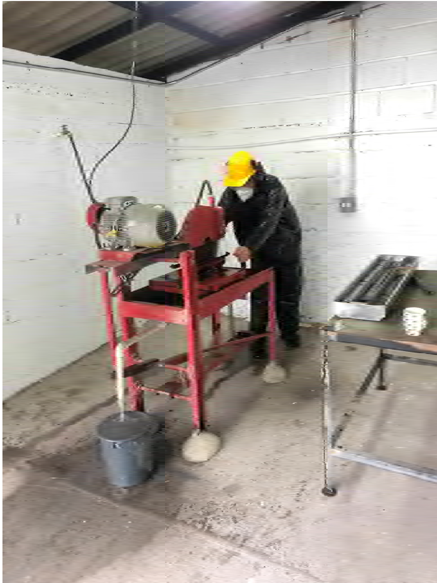
Figure 12-8 Technician demonstrating core cutting procedures. (Source: Mauricio Castañeda, June 12, 2021)
