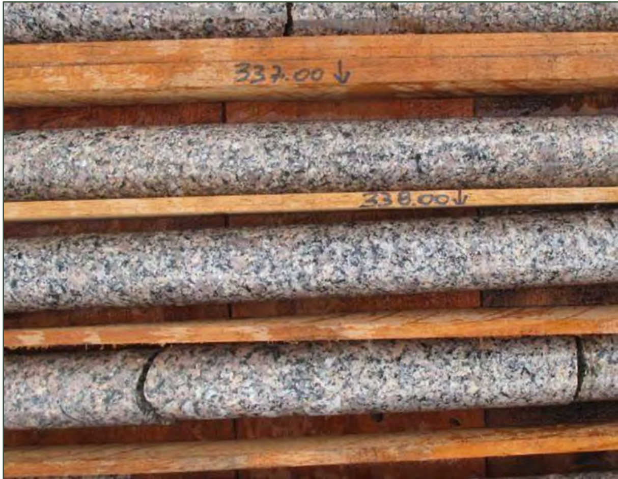
Figure 7-4: Example of Fresh, Un-altered Monzogranite
