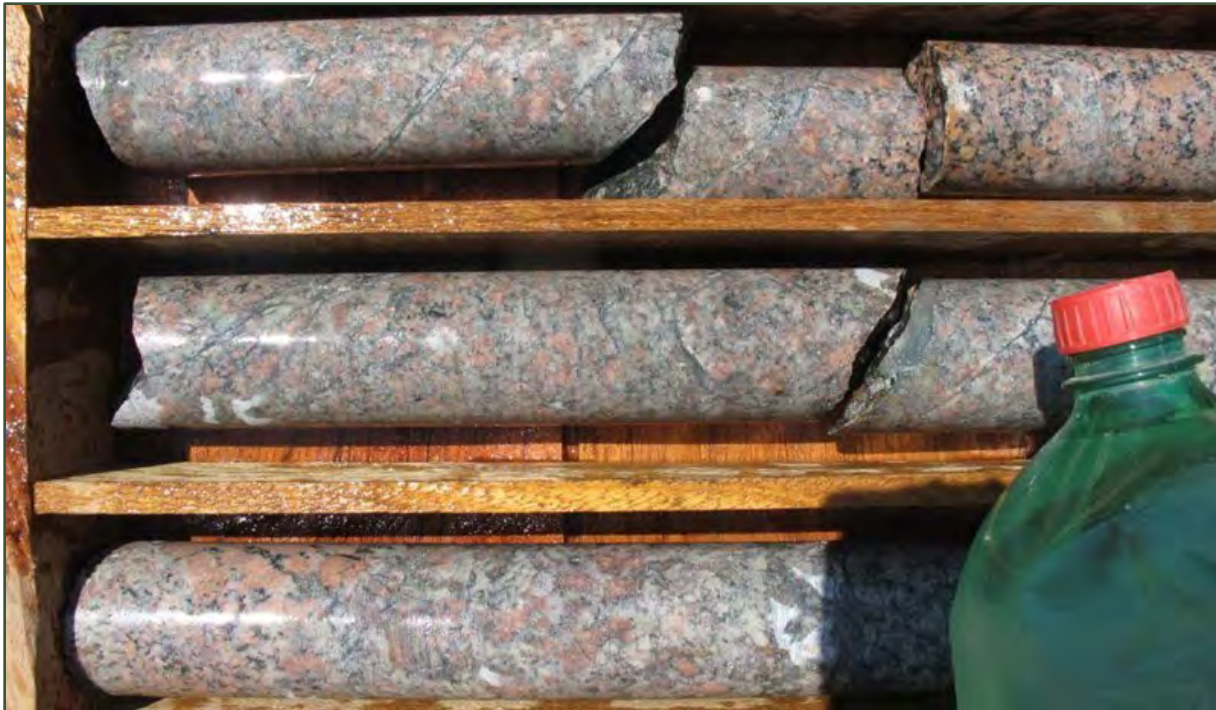
Figure 7-7: Example of Mixed Zone Alteration Type
