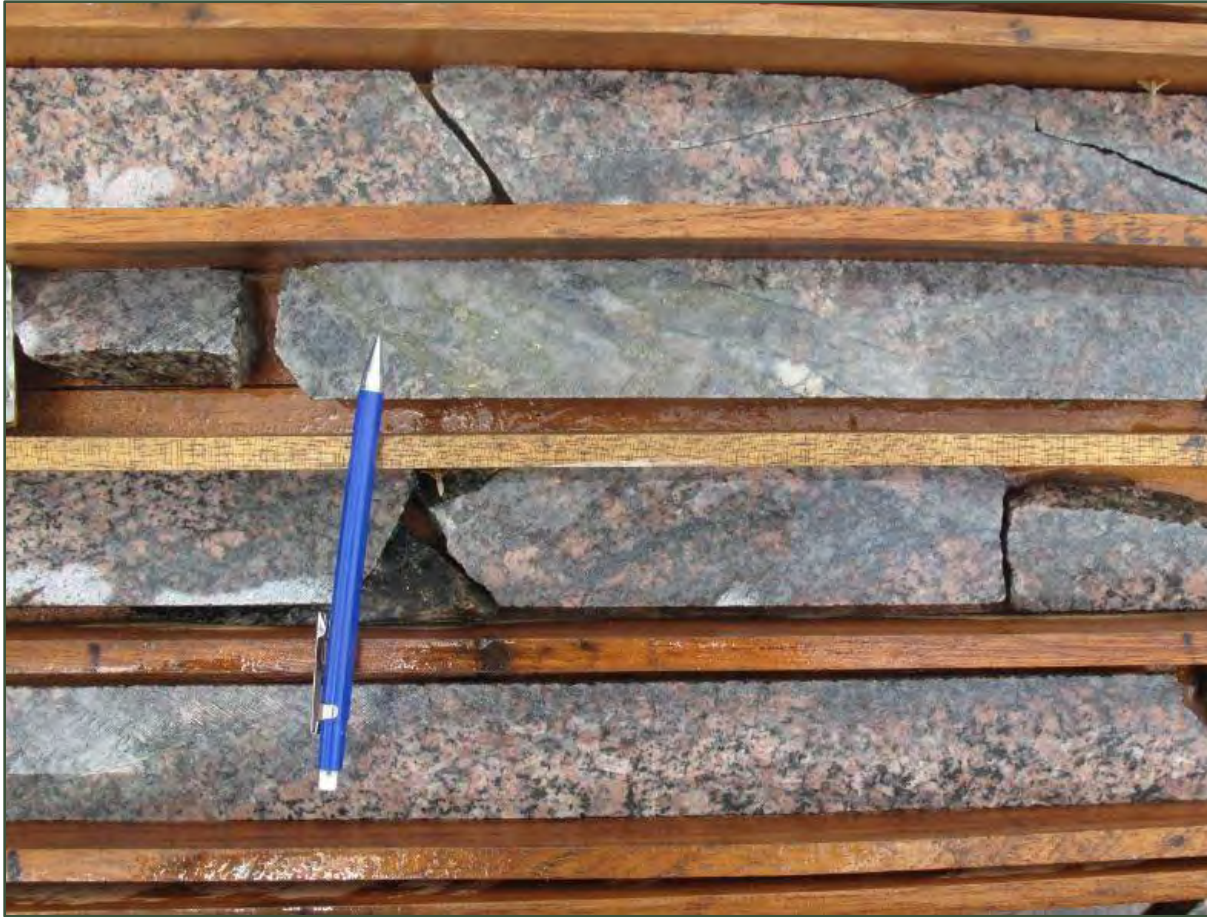
Figure 7-8: Example of Heterogenous Alteration Type Zone
