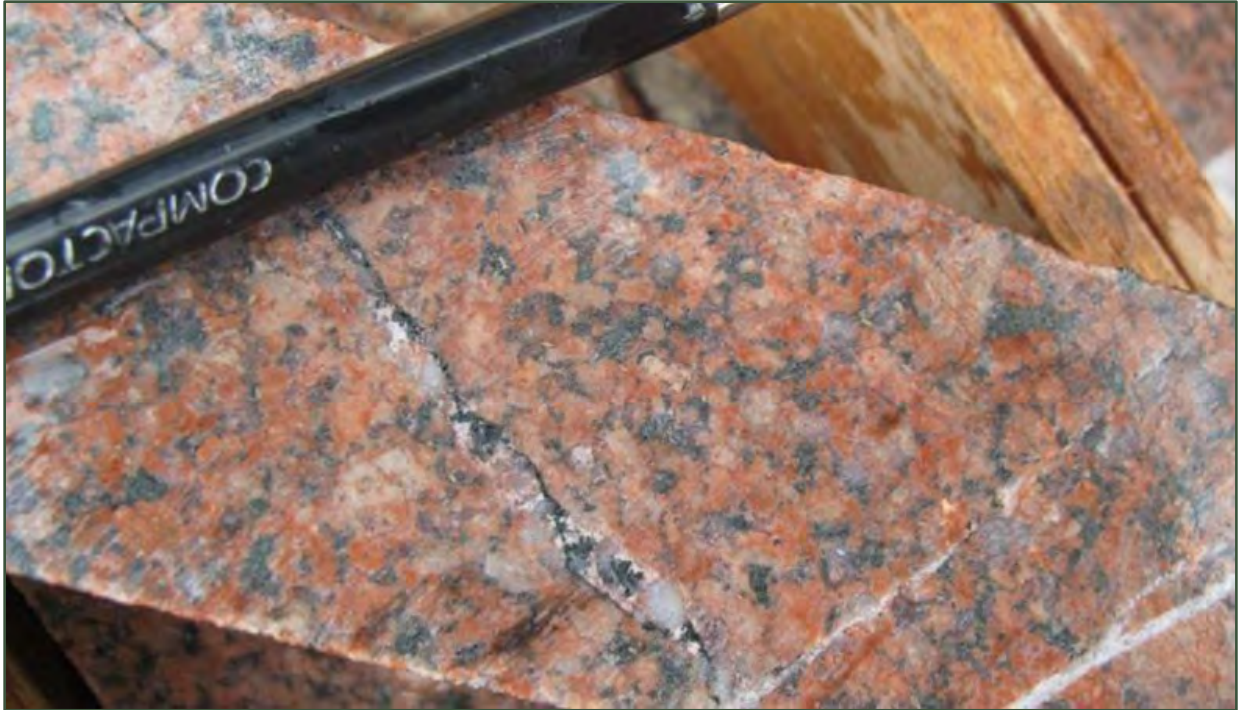
Figure 7-5: Example of Fe-oxide +/- Chlorite Alteration
