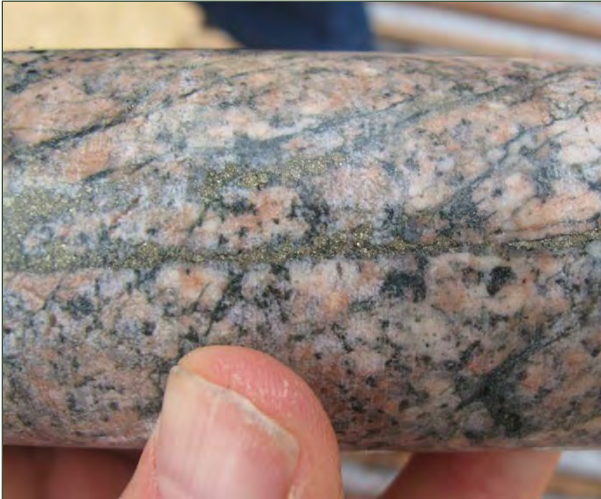
Figure 7-13: Example of Fracture Controlled Vein-Style Pyrite Mineralization within the Fe-Ox-Chlorite Alteration Zone
