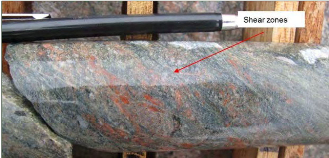
Figure 7-9: Example of a Small Scale Shear Zone in Drill Core
