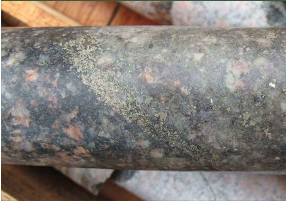
Figure 7-12: Example of Fine Disseminated Pyrite Mineralization within the Mixed Alteration Zone
