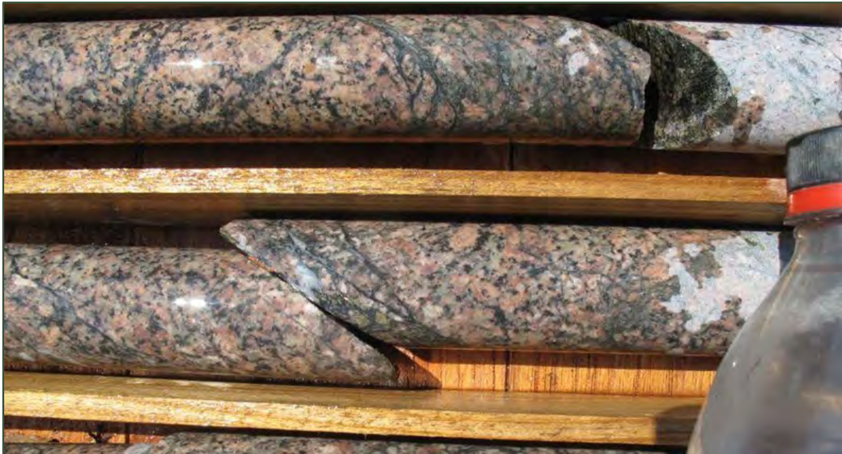
Figure 7-6: Example of K-Feldspar-Epidote-Chlorite Alteration
